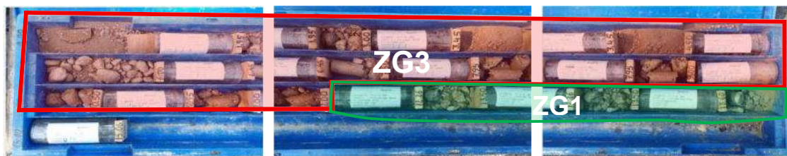
Figure 3 – Sample collected from a borehole drilled at the substation level.
